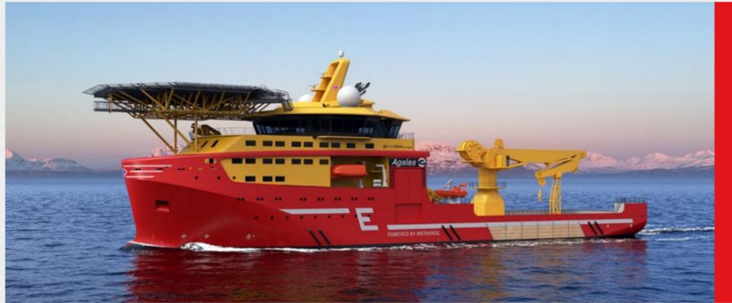
In 2024 Eidesvik announced the construction of a state-of-the-art Construction Support Vessel (CSV) to perform subsea and renewables operations. Equipped with methanol engines and a battery hybrid system the vessel will be among the world's most environmentally friendly vessels within its operating segments.
